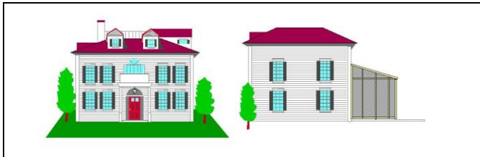
Figure 9 Add on screened porches with metallic frames need bonding to prevent shocks from electrical faults that occur when screws fastening aluminum track to the wall pierce wiring inside the wall and energize the framework.
