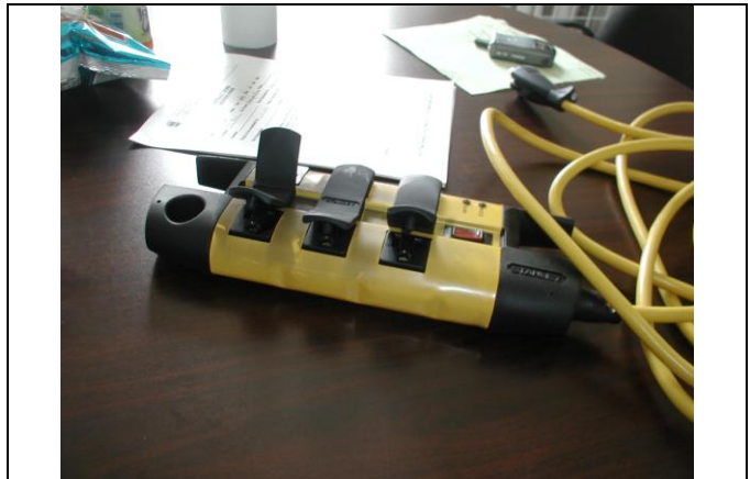
Fig 17 Cheap consumer grade devices with TVSSs not conforming to UL-1449 may initiate collateral fires when their MOVs burn up due to electrical fault such as an open Neutral lead or end of life.
