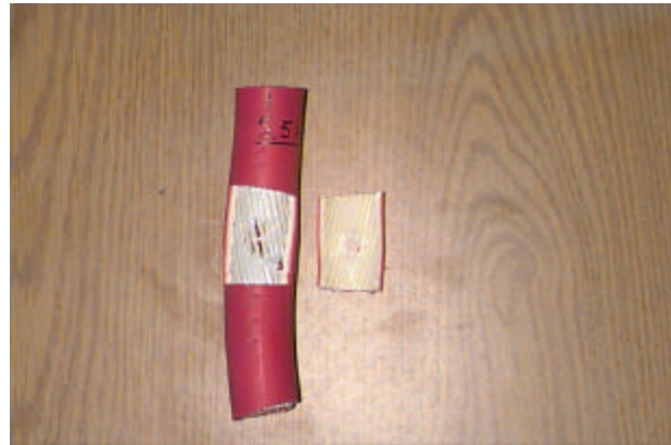
Cutaway of Plastic Insulated B-Strand Cable Showing Typical Strand Displacement
