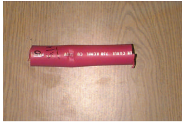
Plastic Insulated B-Strand Cable After Tests
