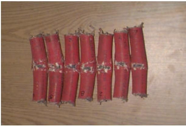
Textile-Covered RHW Following Tests
