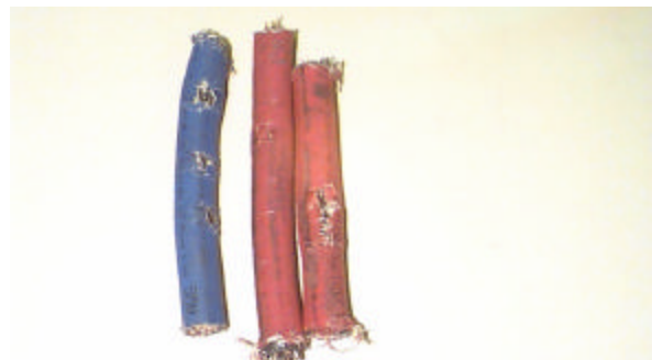
Compression Tests of New Generation Cloth Insulation 350 MCM Power Cable (left and right) and Point Penetration Tests (center).
