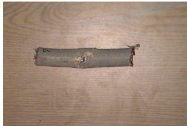
I-Stranded Cable Tends to Flatten Out Under Mechanical Load, Forming a Supportive Bed. Accordingly, the Insulation on I-Stranded Cable Can Tolerate More Than 200% Weight Than B-Stranded Cable.
