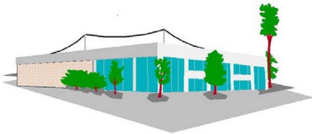
Figure 13 Placing one or more catenary wires on a rooftop is an inexpensive yet reliable way to provide lightning protection for a large rooftop photovoltaic installation.
