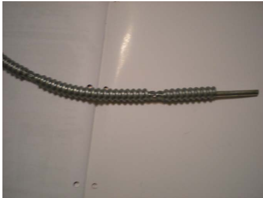
Figure 4 Crimped, armored #2 AWG BTCU wire.
