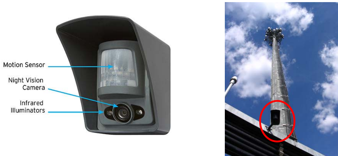
Figure 16 a motion detecting camera that reports events over the cellular network.
