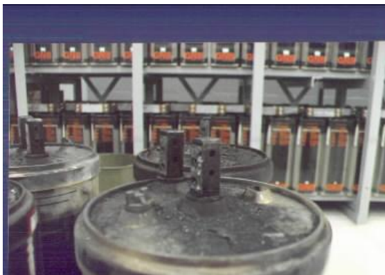
Figures 5 and 6. Post meltdown damage.
