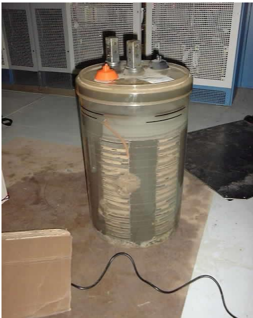
Figures 7 and 8. Severe cell sulphation.
