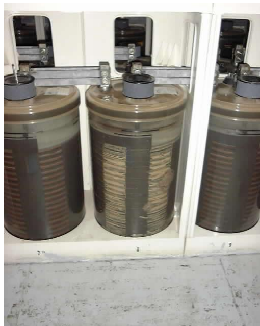
Figures 7 and 8. Severe cell sulphation.
