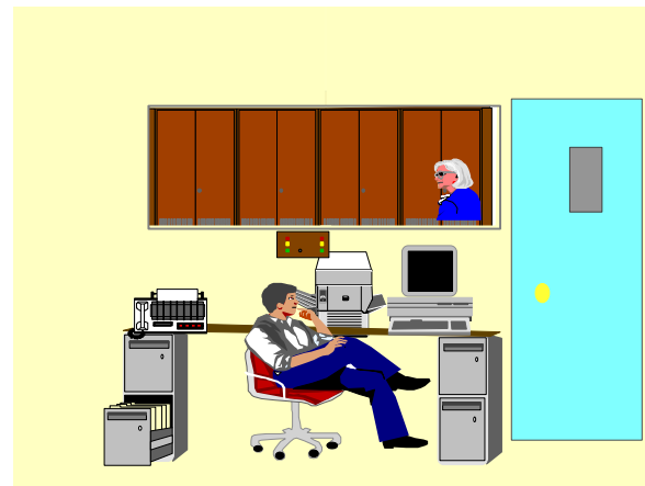
Figure 4 A partition between switching systems and Maintenance & administrative area improves reliability and fire safety by isolating several heat, fuel and contamination sources.
