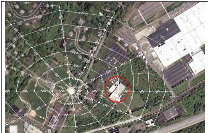
Figure 2 Example of soil resistance from Fig 1 overlaid on an aerial view of a central office (circled) and the surrounding area. The lightning strike potential will divide across the series-parallel voltage divider network placing a significant difference of potential between one side of the building and the other.
