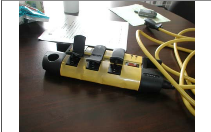
Fig 7 Cheap consumer grade devices with TVSSs not conforming to UL-1449 may initiate collateral fires when their MOVs burn up due to electrical fault or end of life.
